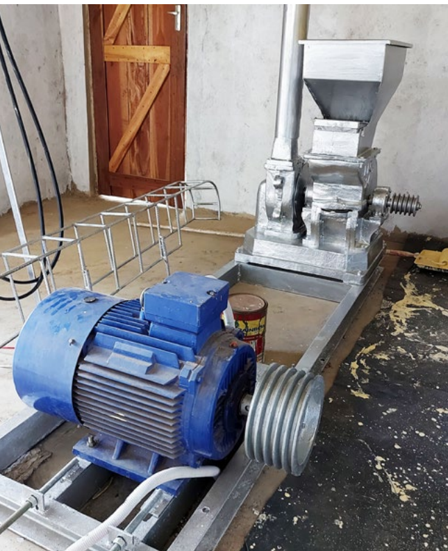
Hopper and electric motor assembly. Kuwala_2023.
